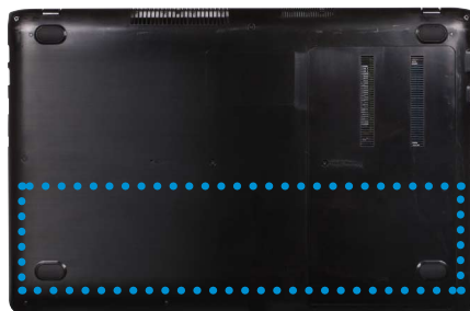
The location of the internal battery
